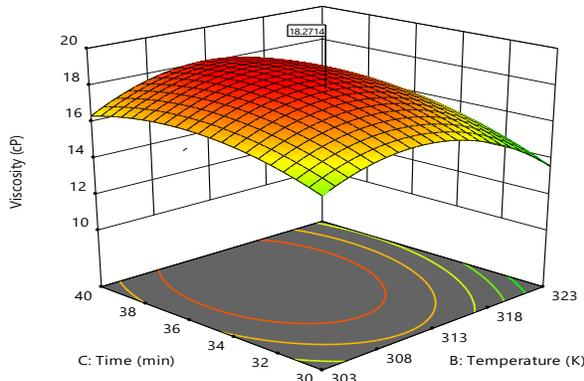
Figure 3: Temperature and time influence on the mud's Viscosity
