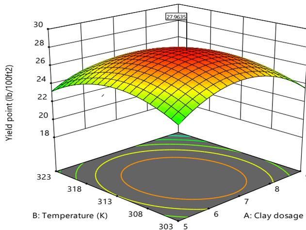
Figure 4: Clay dosage and temperature influence on the mud's yield point
