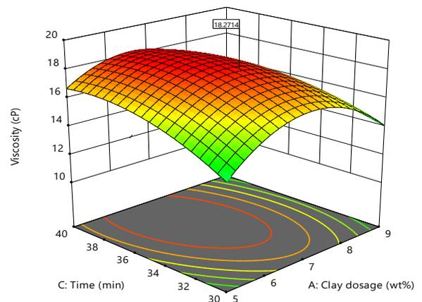
Figure 2: Clay dosage and time influence on the mud's Viscosity
